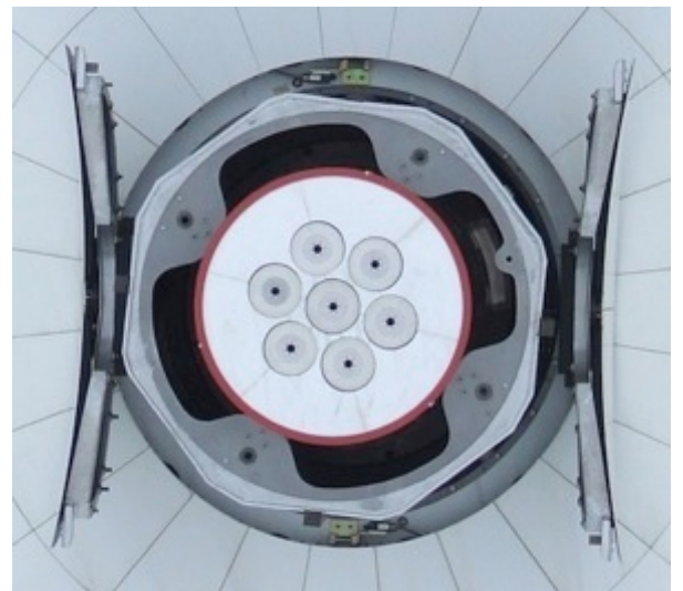
View onto the 7-beam receiver mounted in the prime focus, as viewed from the secondary focus.
